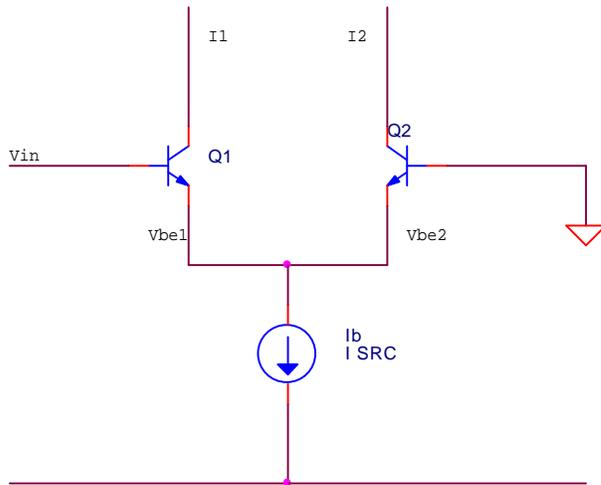
The above figure shows a basic differential pair. So, we can start by writing the following equations:
