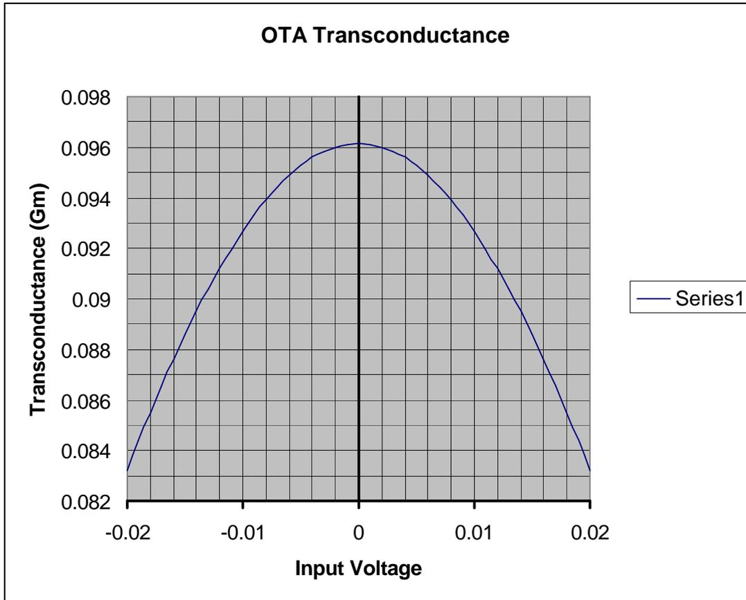
The two above plots show how GM of an OTA will vary with input voltage. The second plot is just more magnified around 0 volts which is where they are generally operated. What you will not is that even when the input range is limited to +/- 10mV, GM has already changed by 3% to 4% (closer to 3%). To keep the linearity to within 1%, you need to limit the input to +/- 6mV.
